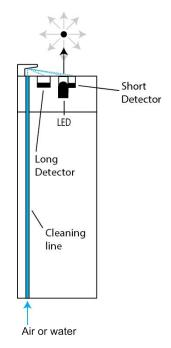
can be used to detect low and high concentrations of solids. The SoliSense® uses Pi's novel measurement technique that automatically takes readings at four different light levels and uses the gradient between the four readings to produce the sensor output. This configuration allows accurate and reliable measurements of suspended solids concentrations and turbidity to be made.
