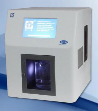
LE100 liquid particle counter (updated from model L01A-24) is mainly used for detection of insoluble particles in injection, infusion, sterile powder under USP <788> "Particulate Matter in Injections", and particle contamination detection of infusion equipment, anesthesia equipment, medical packaging materials. It can also be used for particle detection in organic, colored and transparent, oil-based liquid samples.
